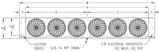
**NOTE**: Refrigerant and electrical connection locations have been changed for the Next-Gen All-Temp design. Standard connections are now opposite of the legacy All-Temp models.
